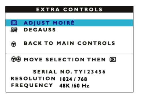
4) Press the button. The ADJUST MOIRE window appears. HORIZONTAL will be highlighted, press to confirm.
